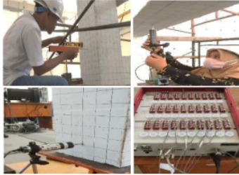
Figure 6. LVDT on test pieces and installation photos
