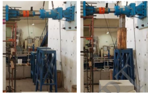
Figure 4. Cyclic testing equipment setup
